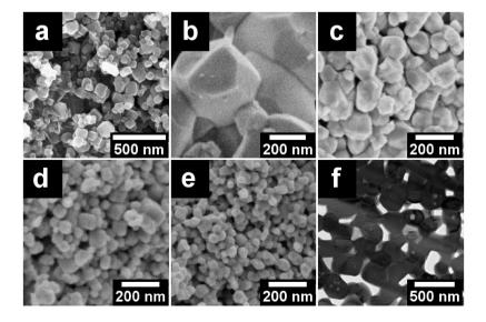
Figure 3. SEM images of (a) as prepared nanoparticles, (b) conventionally treated sample (CS), (c, d, e) samples treated under the exposure of 300, 600 and 900 V/cm, respectively; (f) TEM image of a lamella cut from sample FS\_600 with a focused ion beam, showing the porous structure of the materials.
