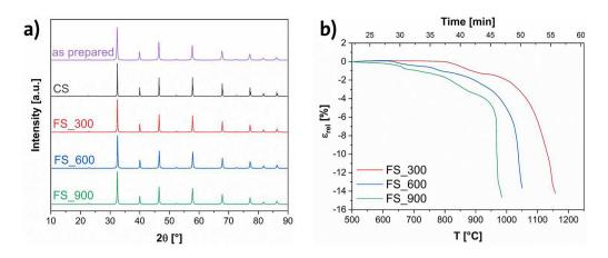
Figure 1. (a) X-ray diffraction patterns of the as prepared and high temperature treated SrTiO<sub>3</sub>. (b) Plots of the linear shrinkage against the furnace temperature during the electric field assisted treatment.
