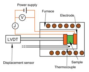
Figure 2. Schematic representation of the setup for the electric field assisted treatments.
