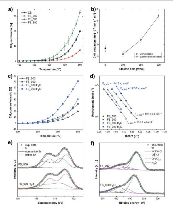
Figure 6. (a) Light-off curves obtained from the methane oxidation experiments. (b) Reaction rates at 700 °C normalized by the BET surface area. (c) Light-off curves and Arrhenius plots of the reaction rate (d) of FS\_600 and FS\_900 samples before (grey) and after (blue) hot water treatment. Sr3d (e) and O1s (f) XPS spectra of SrTiO<sub>3</sub> exposed at 900 V/cm before (FS\_900) and after (FS\_900 H<sub>2</sub>O) hot water treatment.
