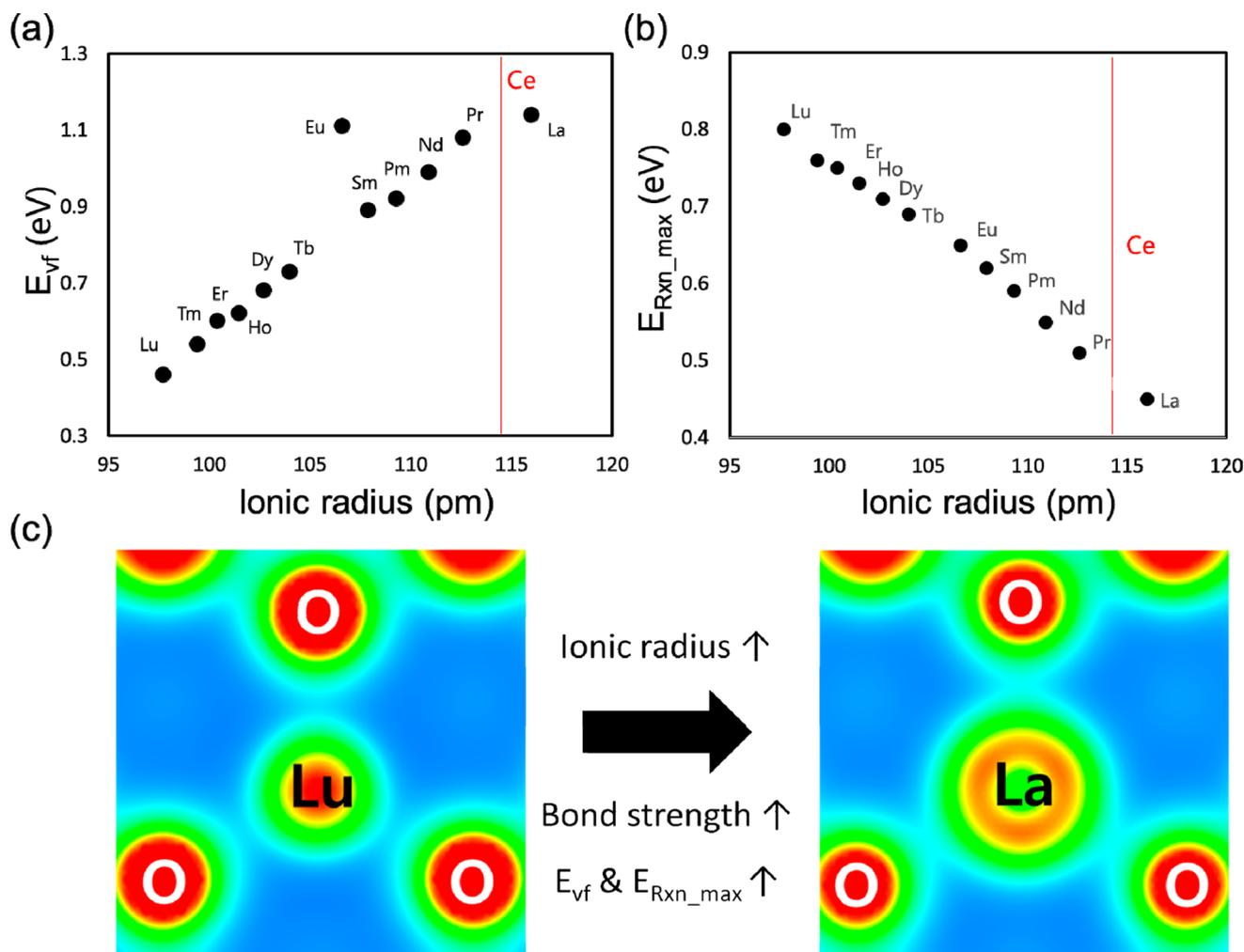
**Figure 4.** Linear relationships between (a) oxygen vacancy formation energies or (b)  $E_{Rxn\_max}$  and the ionic radius of dopants on RE-doped  $CeO_2(111)$ . (c) Charge density distribution of RE dopants with the smallest (Lu) and the largest (La) ionic radius bonded with the NN oxygen atoms in RE-doped  $CeO_2(111)$ .
