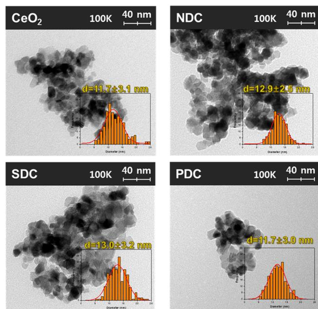
**Figure 1.** TEM images and particle size distributions of doped ceria NPs.
