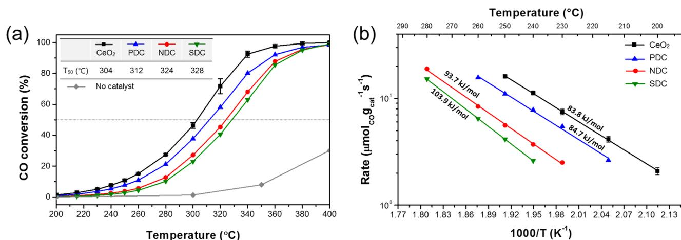
**Figure 2.** (a) Light-off plots for CO oxidation over doped ceria NPs. (b) Arrhenius plots for CO oxidation over doped ceria NPs. The activation energies are indicated above each line.
