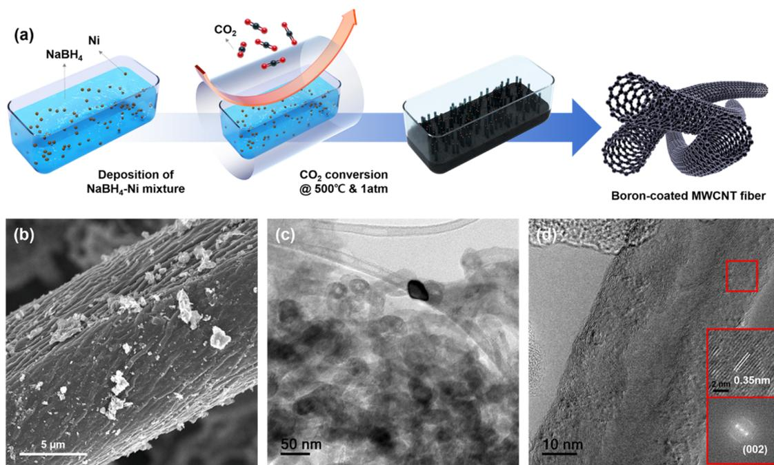
**Figure 1.** (a) Schematic illustration for the synthetic route of the CB-CNT based on  $\text{CO}_2$ -based CVD. (b) SEM image of the CB-CNT. (c) TEM image of the CB-CNT and (d) its high-magnification version [insets: FFT pattern and interlayer spacing of carbon (002)].
