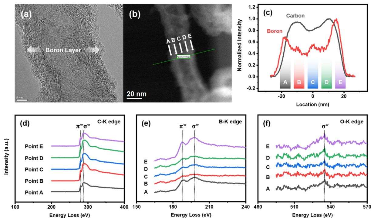
**Figure 2.** (a) HRTEM image. (b) Scanning TEM image of the CB-CNT to obtain the EELS spectra (the green line indicates the location for the EELS line profiling). (c) Overlay of the carbon and boron signals from the EELS line profiling depending on the location. (d–f) EELS spectra of each element depending on the location.
