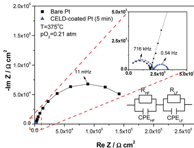
Fig. 5 Typical impedance spectra of bare (black) and CELD-coated Pt (blue) electrodes on both sides of a YSZ single-crystal electrolyte measured at 375 °C with  $pO_2 = 0.21$  atm. A magnified semicircle of CELD-coated Pt electrode at low-frequency is indicated. The impedance spectra were modelled by a series of two parallel RC sub-circuits (insert). Solid line: the fitting results.
