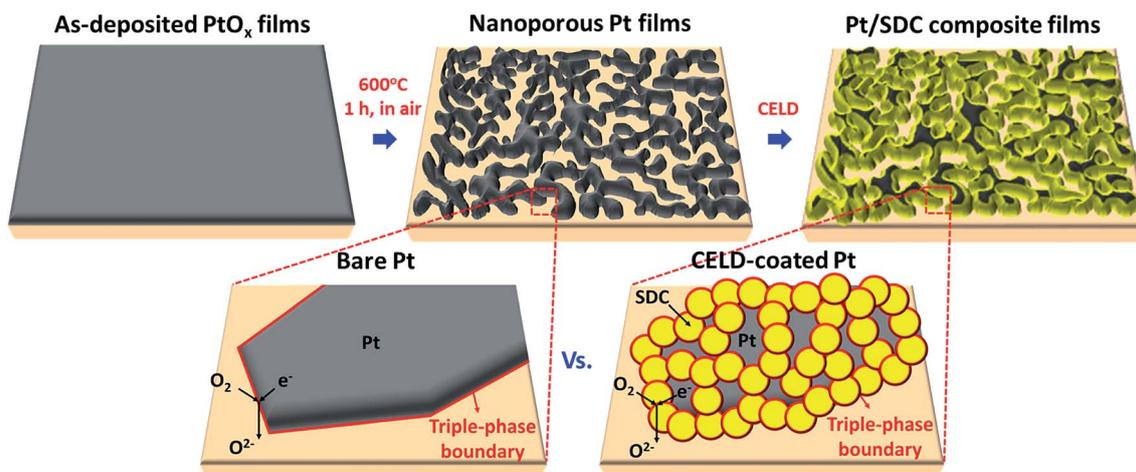
Fig. 1 Schematic diagram of the overall fabrication procedures (top) and the targeted structure of composite films in this work, compared to bare Pt (bottom). SDC: Sm<sub>0.16</sub>Ce<sub>0.84</sub>O<sub>1.92- $\delta$</sub> .
